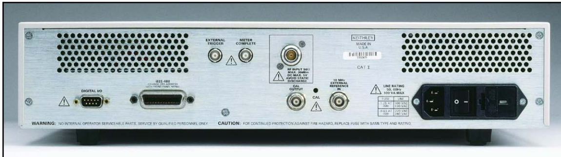
Figure 8. Rear panel of 2800 showing Type N input connector, external reference input, calibration output, external trigger and measurement complete BNC connectors, IEEE-488 connector, and DB9 digital I/O relay control lines connector.
